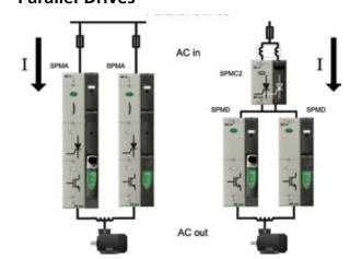
For higher currents multiple SPMAs or SPMDs may be configured in parallel. The SPMA may give shorter installation time with less interconnections but the SPMD may give lower cost. Site standardization may also be a factor.
